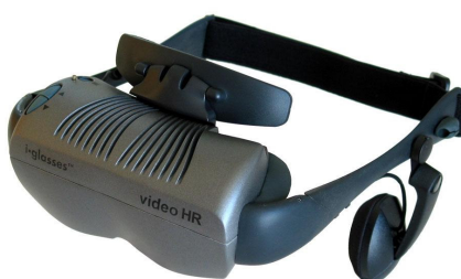
FIGURA 2.2. HMD I-GLASSES DA I-O DISPLAY SYSTEMS (ABSOLUT, 2007).
