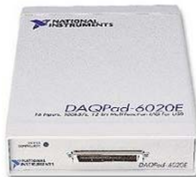
FIGURA 31 - CONVERSOR A/D DAQ PAD 6020E
