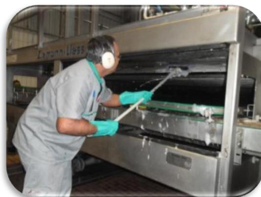
*FIGURA 21: PASSO 1 DA MA – LIMPEZA DA MÁQUINA.*
